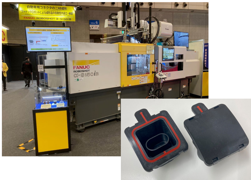
Two components molding products of automotive waterproof connectors
