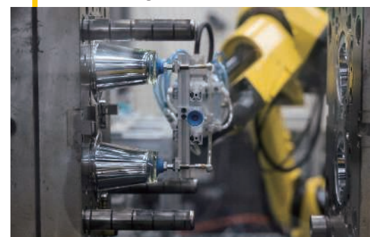
Plastic molding with ROBOSHOT
