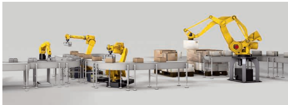
Image - Picking, packing, and palletizing processes utilizing robots
