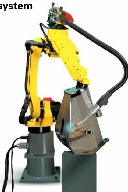
Bracket part arc welding system
