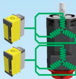
2. Driving large motor by "Multi Amplifiers Drive"
