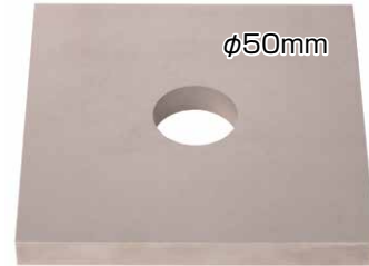
Die steel, 20mm 1 rough 5 skims Roundness 0.90 \mu m
