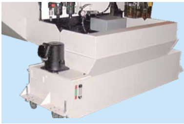
Coolant unit (tank)
