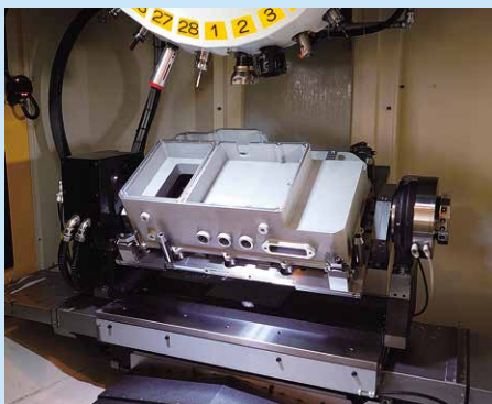
Example of indexing application by DDR-TiB
