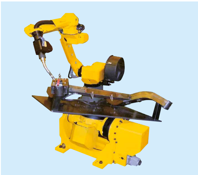
Automobile part arc welding with Servo Torch
