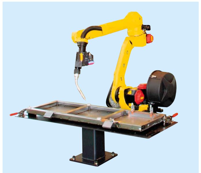
Architectural part arc welding with i RVision
