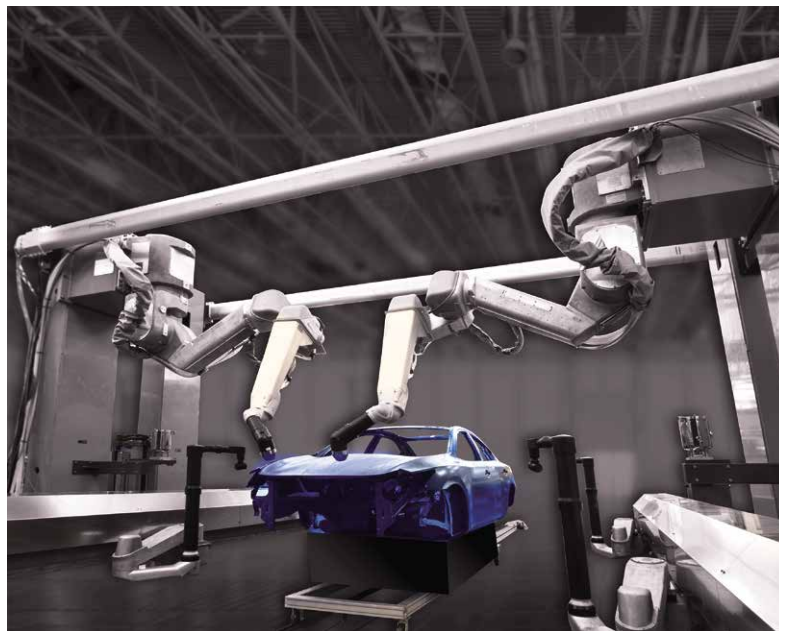
Body painting by P-1000iA and door opener P-20iB
