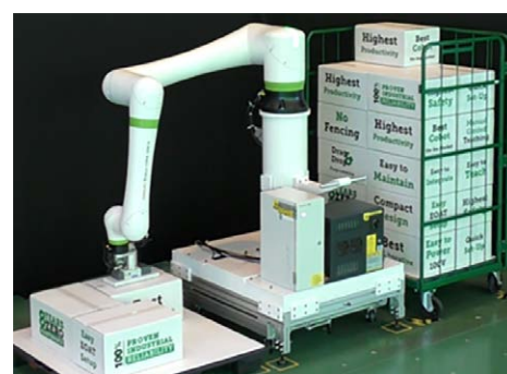
Palletizing by a CRX-25iA (The photo shows the area around the singular point when the wrist is fully extended.)
