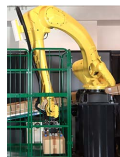
Palletizing by a M-710iD/50M (The photo shows the area around the singular point when the wrist is fully extended.)
