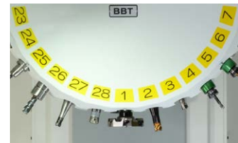
Turret with a tool storage capacity of 28 tools
