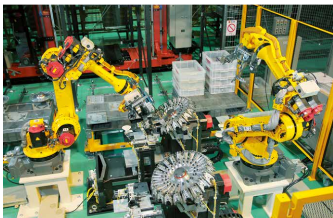
工具交換機構の組立て Assembly of automatic tool changers
