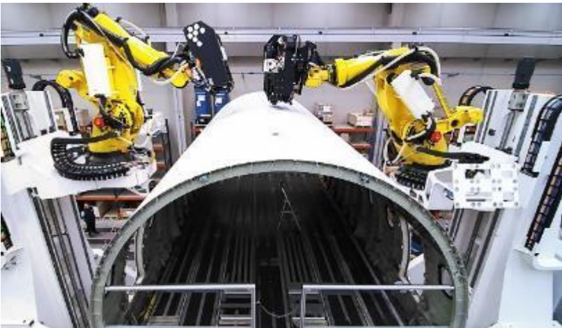
Drilling in aircraft bodies
