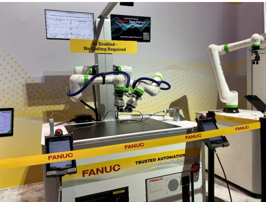
Dual-Arm CRX-5iA Connector Assembly
