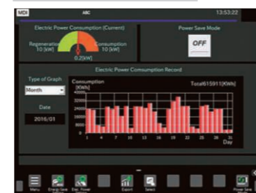
Energy saving screen provides energy saving settings manager of machine and optional equipment and energy consumption monitor.
