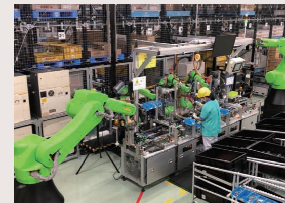
Full view of the system (one worker and five robots)
