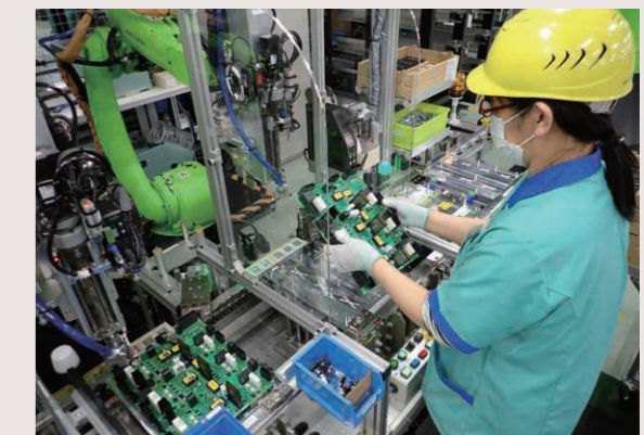
Positioning parts (by the worker) and tightening screws (by the robot)
