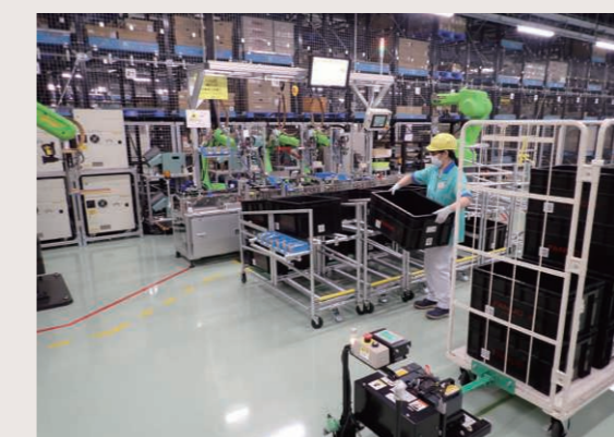
Delivering parts with an automated guided vehicle
