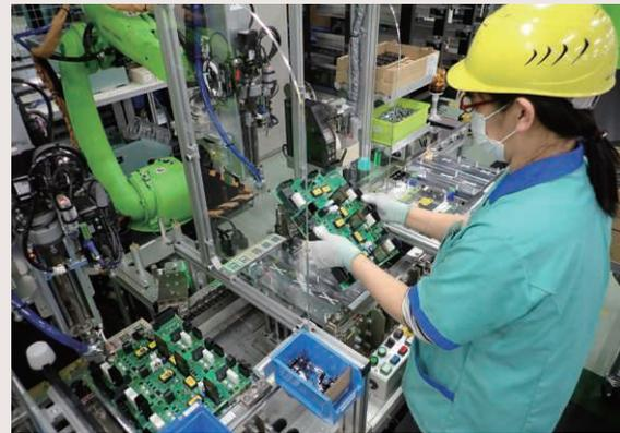
Positioning parts (by the worker) and tightening screws (by the robot)
