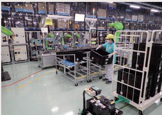
Delivering parts with an automated guided vehicle
