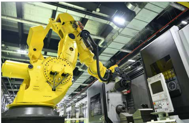
Cell for machining large parts using a large size robot
