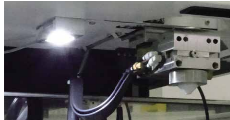
High-brightness LED (Left side of work tank)
