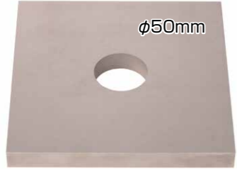
Die steel, 20mm, \phi 0.25 brass wire 1 rough 5 skims Roundness 0.90 \mu m
