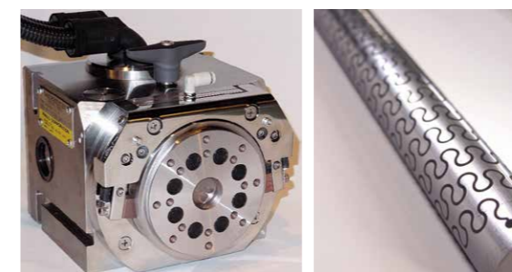
High precision positioning, light weight, and compact rotary table
