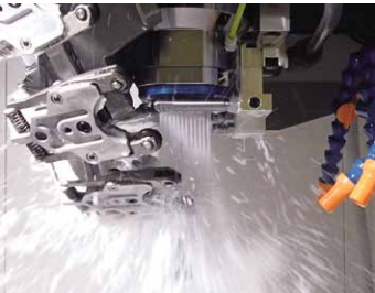
Taper cleaning function Tool taper and spindle taper are washed with coolant during tool change to reduce chips getting caught.
