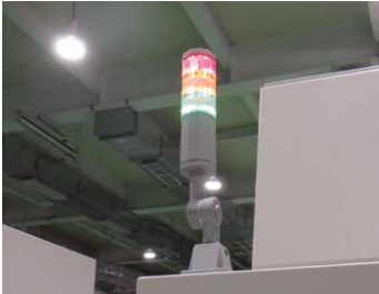
Signal lamp (3 colors) LED type lamp of long-life and energy-efficient. It can be tilted in any direction to suit the machine layout.
