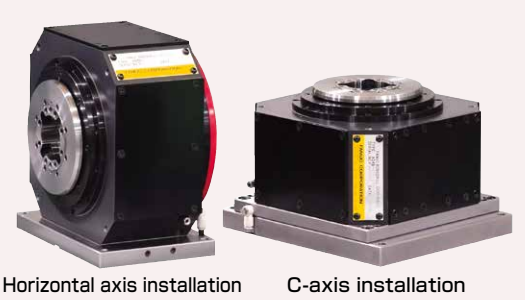
DDR-HSiB High-speed rotation type unit capable of turning, in addition to high-speed and high-precision positioning. The installation direction can be selected according to the application. Max. rotation speed: 1,500min -1
