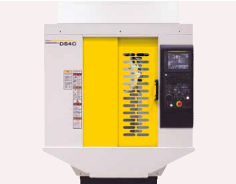
Wide open front door Changing large workpiece or fixture becomes easier. Opening width: 730mm (D54C)/1095mm (D74C) *not available for D116C
