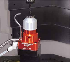
Tool length measurement switch Highly reliable type with overtravel detection. Multi-function measurement macro program is also included as standard.
