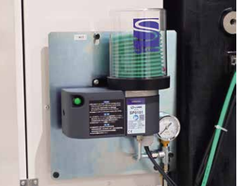
Automatic grease lubrication Automatic lubrication to XYZ axis guides and ball screws is changed from oil type (standard) to grease type, that consumes less and has excellent running costs.
