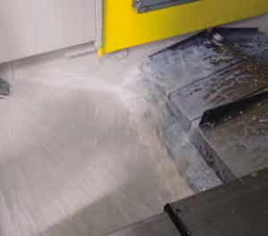
Chip flush function Chips that scatter inside the machine are washed away. The new piping design has significantly improved cleaning efficiency.
