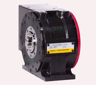
DDRiB/DDR-HPiB Dedicated additional 1-axis rotary table that enables high-speed and high-precision, non-backlash positioning with direct drive motor. Max. rotation speed: 300min -1
