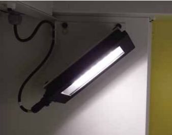
Illumination (LED type) High-brightness LED is applied and installed on the back of the operation panel.
