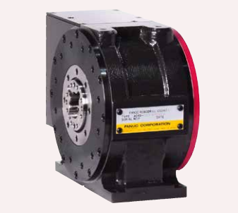
DDRiB Dedicated additional 1-axis rotary table that enables high-speed and high-precision, non-backlash positioning with direct drive motor. Max. rotation speed: 300min -1
