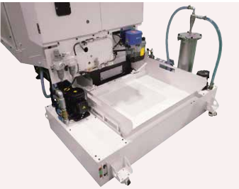
Coolant unit (tank) Selectable between 260L type (photo) on which center-through pump unit can be equipped, and the compact 120L type.
