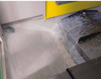
Chip flush function Chips that scatter inside the machine are washed away. The new piping design has significantly improved cleaning efficiency.
