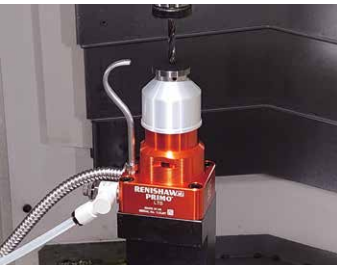
Tool length measurement switch Highly reliable type with overtravel detection. Multi-function measurement macro program is also included as standard.
