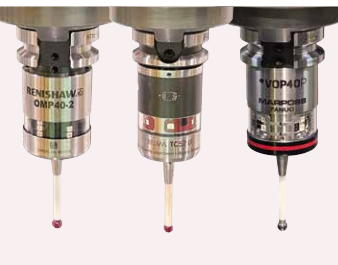
Touch probe Can be used for workpiece centering and thermal displacement compensation. Infrared communication type and radio communication type are available.
