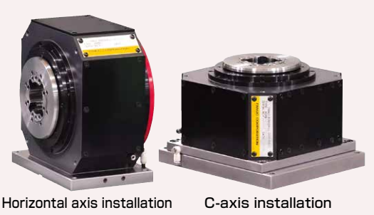
DDR-HSiB Horizontal axis installation C-axis installation High-speed rotation type unit capable of turning, in addition to high-speed and high-precision positioning. The installation direction can be selected according to the application. Max. rotation speed: 1,500min -1
