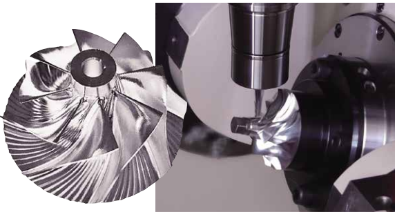
High-speed machining of impellers using a 2-axis DD motor rotary table
