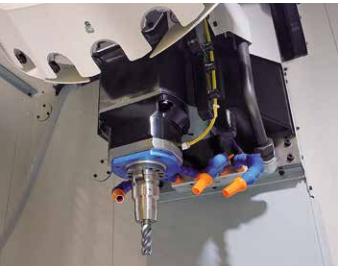
Coolant unit (nozzle) Coolant is surely delivered to the cutting point by 4 nozzles even tool lengths are different. Interference is reduced by running the piping inside the spindle.
