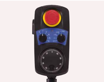
Portable manual pulse generator When working away from the operator's panel such as setting up jigs, it makes easier to operate each axis. Comes with a magnet on the back.
