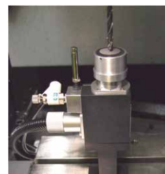
Tool length switch for automatic measurement
