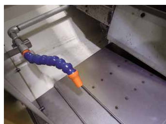
Coolant unit with chip flush (spot gun provided)
