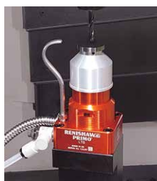
Tool length switch for automatic measurement
