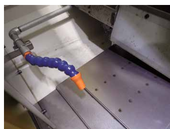
Coolant unit with chip flush (spot gun provided)
