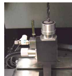
Tool length switch for automatic measurement
