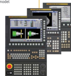
ROBOSHOT α-SiB [2021] Excellent operability with a display unit having the largest screen in the industry and an original dual-screen simultaneous display function.
