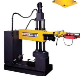
FANUC ROBOT MODEL 1 [1977] Developed as FANUC's first robot product. Cylindrical coordinate type with simultaneous single axis control.
