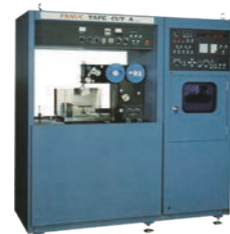
FANUC TAPE CUT-SERIES A [1975] FANUC developed an electric discharge machine in order to spread the use of NC machine tools.
