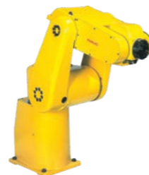
LR Mate [1992] ROBOT for loading and unloading workpieces to and from machine tools. The name originates from the abbreviation of "Loader Robot."
