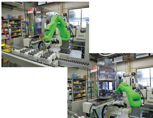
Cylindrical grinding automation system using the CR-7iA
