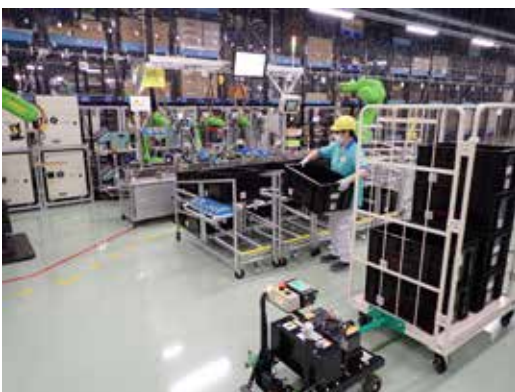
Delivering parts with an automated guided vehicle
