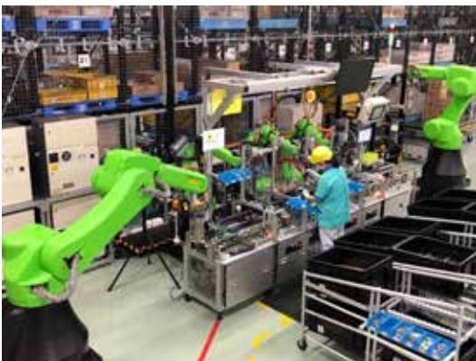
Full view of the system (one worker and five robots)
