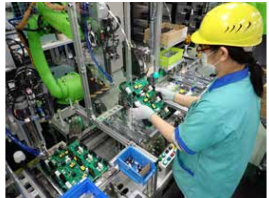
Positioning parts (by the worker) and tightening screws (by the robot)
