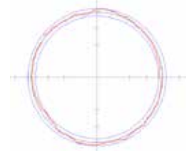
50 mm hole diameter in 20 mm thick die steel material Example of cutting a true circle
