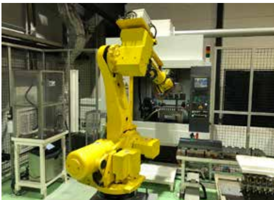
Column machining process (The robot supplies column checked with vision sensors to the ROBODRILL.)
