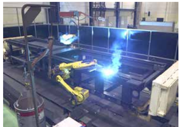
Welding process (Two robots weld the base frame on the turnover device.)
