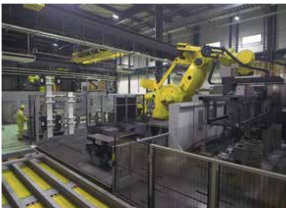
Top surface machining process (The super heavy payload robot sets the base frame up on the machining jig.)
