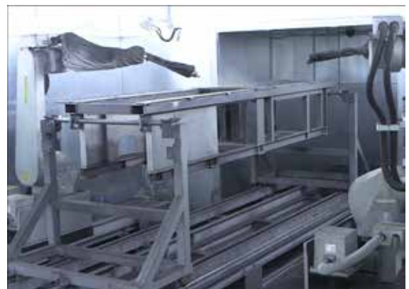
Painting process (Two robots give the base frame a high-quality paint job.)
