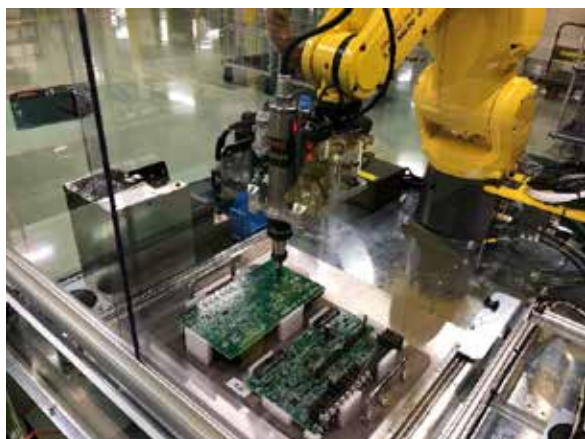
Robot module fastening screws on a PCB
