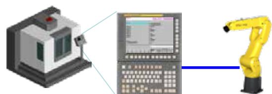
Connecting the CNC and the robot with only one Ethernet cable
