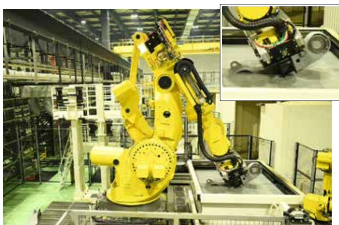
Washing by a robot by dipping in water
