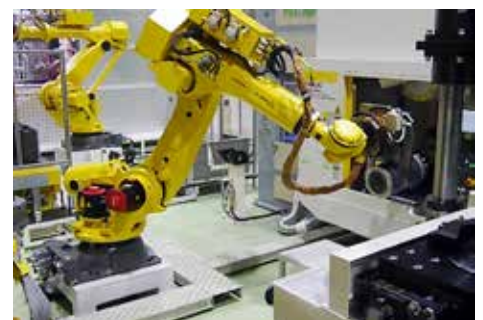
Machining the sprue cut opening with a ROBODRILL
