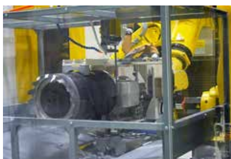
Cutting the sprue of the cast workpiece with a general-purpose bandsaw
