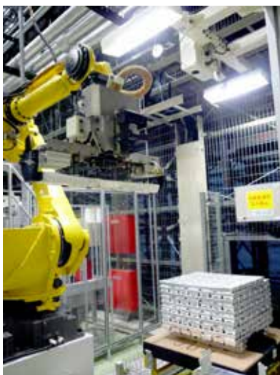
Detecting and unloading ingots using 3D area sensors
