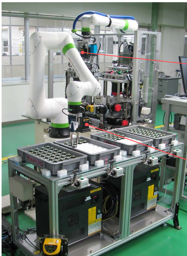
Signal adjustment system for the small \beta i Pulsecoder using the collaborative robot CRX-10 i A
