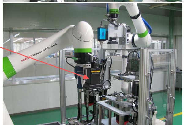
Signal adjustment system for the small \beta i Pulsecoder using the collaborative robot CRX-10 i A
