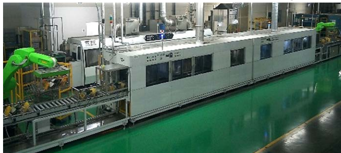
Two collaborative robots that load and collect repair products and an automatic washing machine
