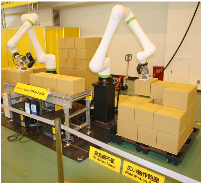
Palletizing with 25 kg payload CRX
