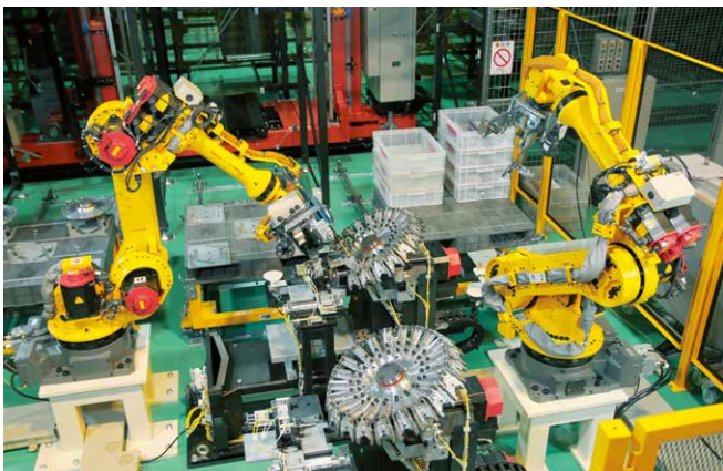
工具交換機構の組立て Assembly of automatic tool changers
